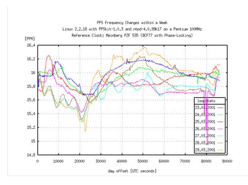
Dave Mill's 2001 experiment on looking at clock stability over a one week period using a Linux PC
