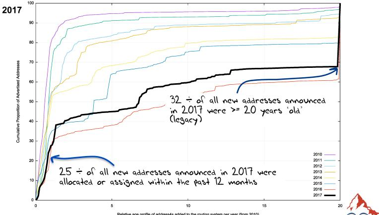
Relative age profile of address4s added to the routing system per year (from 2010)
