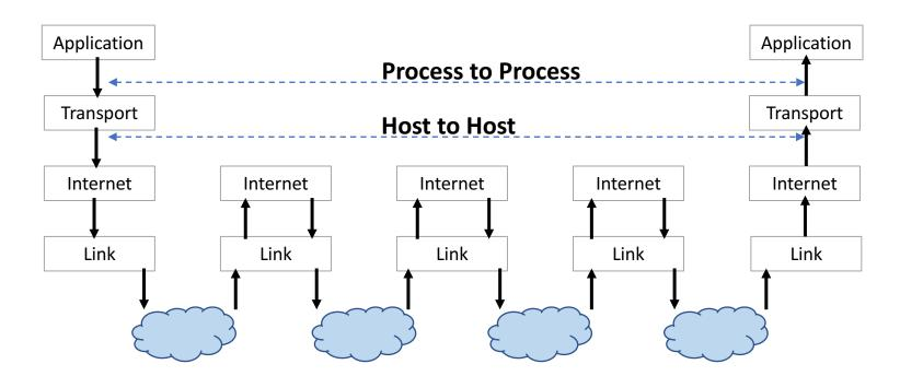
The intention was that only the IP header is used by the network, and the entire remainder of the packet, including the transport headers, is an opaque payload
