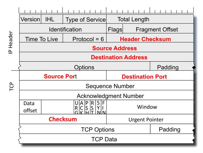
These NATs allow address sharing by using the transport protocol's port fields as part of the address 'distinguisher'
