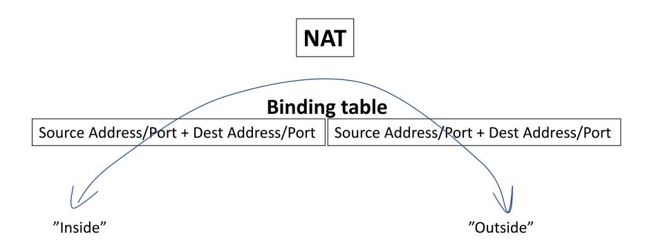
NATs take the 96-bit 4-tuple of Protocol+Address+Ports and replace the packet's fields that match one side of the binding table with the fields on the other side
