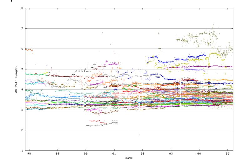
A constantly increasing number of ASNs can be related to average AS path length. The relatively constant AS path length for all AS paths implies that the density of AS interconnection is increasing at a rate proportional to the number of ASNs being added.
