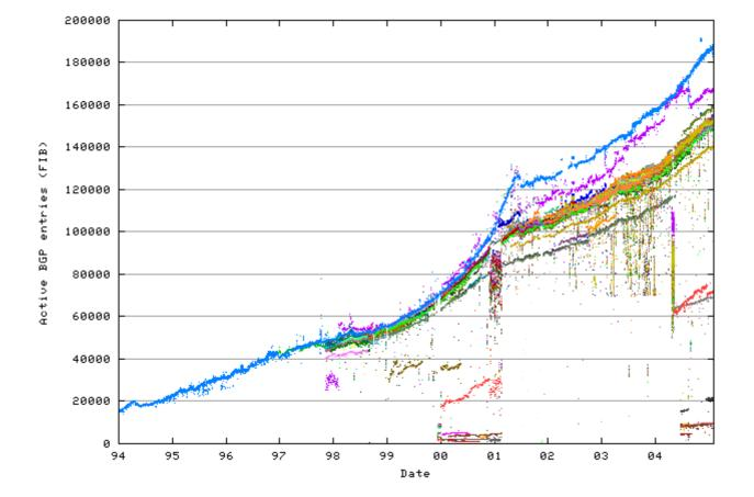
Data assembled from a variety of sources, Including Surfnet, Telstra, KPN and Route Views. Each colour represents a time series for a single AS.
