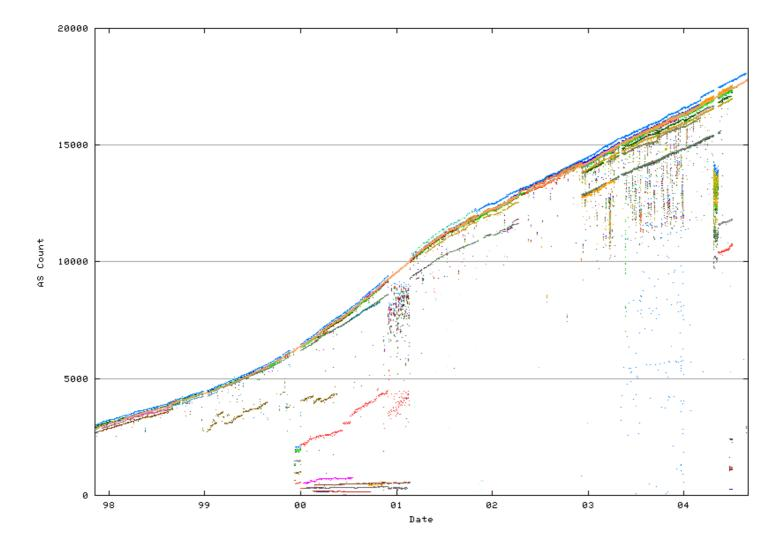
Since early 2001 the number of ASNs in the routing table has been growing at a constant rate, closely matching a linear growth model. New ASNs track the growth of new service providers.
