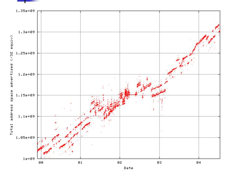
This is the same data for a single AS. It is evident thjast the number of unstable /8 advertisements has dropped from 3 to 1 over this period. It is also apparent that the rate of growth in 2004 is slightly higher than that of 2000.
