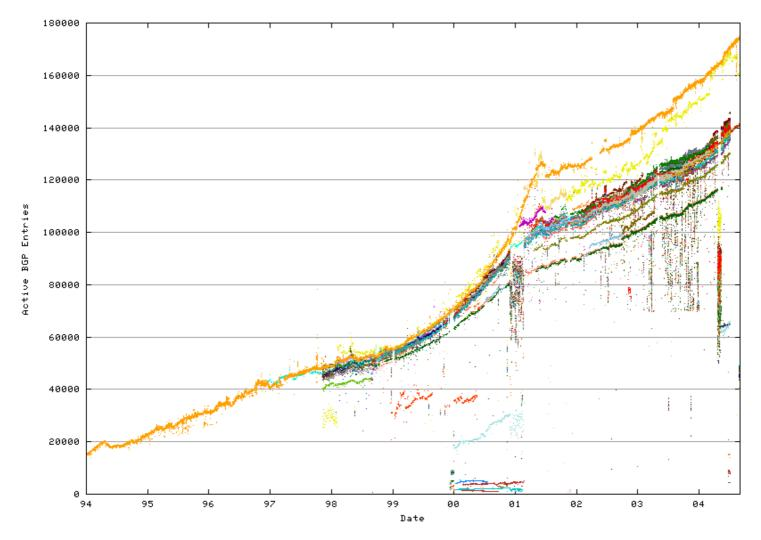
Data assembled from a variety of sources, Including Surfnet, Telstra, KPN and Route Views. Each colour represents a time series for a single AS.
