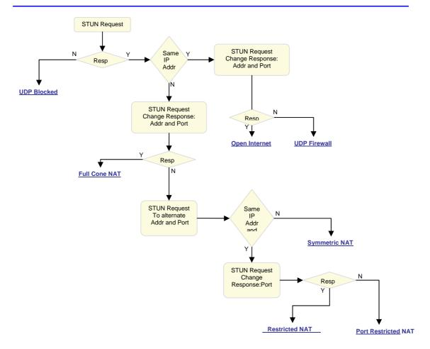
Figure 9 – NAT Discovery Process using STUN
