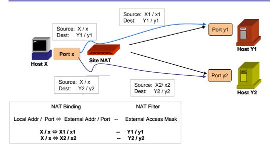
Figure 11 – Outbound connections from a common source
