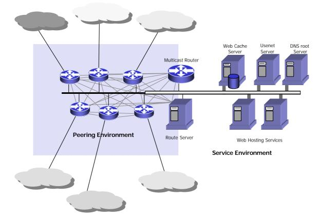
Figure 7. Exchange-located service platforms.
