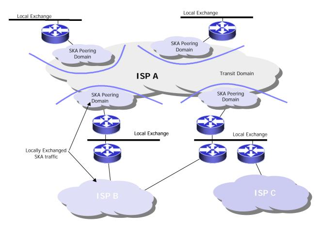
Figure 12. SKA peering using local cells.
